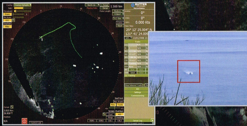
Sigma S6 image of a small craft being tracked by shore based Small Target Detection system. The same craft is otherwise barely visible amongst other surface features.
